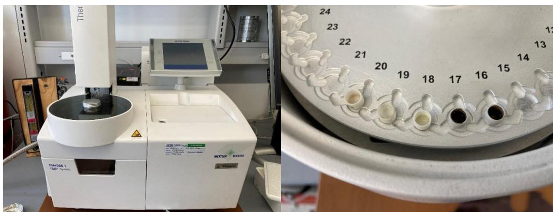
**Fig. A.7.** Left: TGA instrument. Right: crucibles ready for TGA analysis. The crucibles in positions 16 and 17 contain particles already raised to 800°C, whereas the crucibles in positions 18-20 have yet to be analyzed.
