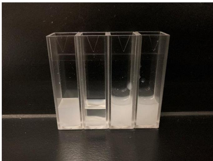
**Fig. B.2.** Qualitative stability test of silica particles. From left to right, the cuvettes contain (1) bare, ungrafted silica in DIW; (2) bare, ungrafted silica in 5API brine; (3) PEG-coated silica in DIW; and (4) PEG-coated silica in 5API brine. The second cuvette, (2), is analogous to case (b) from Fig. B.1.
