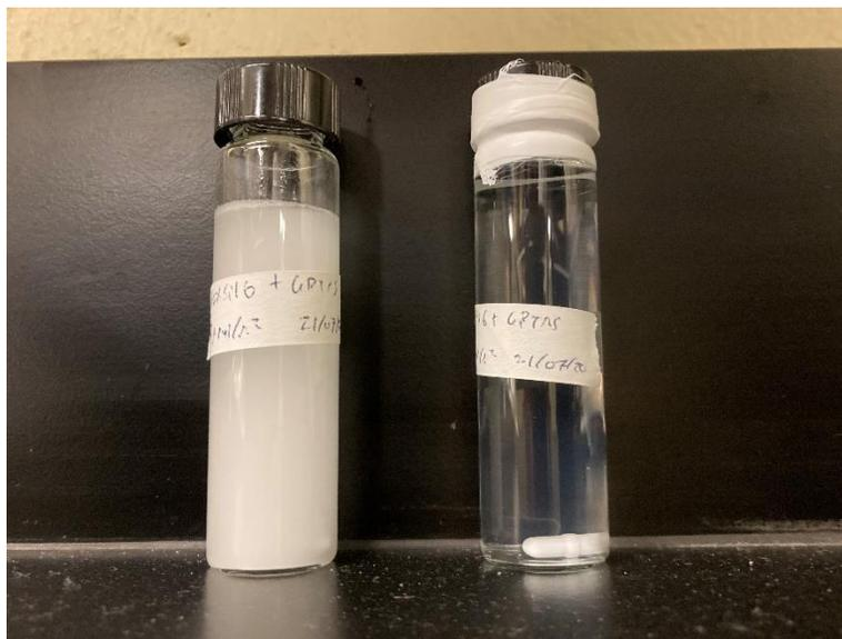
**Fig. A.5.** Left: GPTMS and NexSil 6 reacted without methanol. Right: GPTMS and NexSil 6 reacted with methanol.
