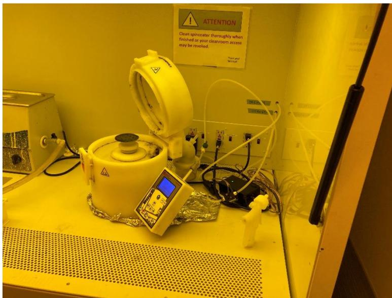
**Fig. B.7.** Laurell WS-650-23 spin-coater. This specific instrument is located inside a class 100 clean room.
