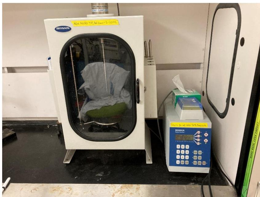
**Fig. C.1.** Branson 450 Digital Sonifier for sonicating oil and water mixtures to form emulsions.
