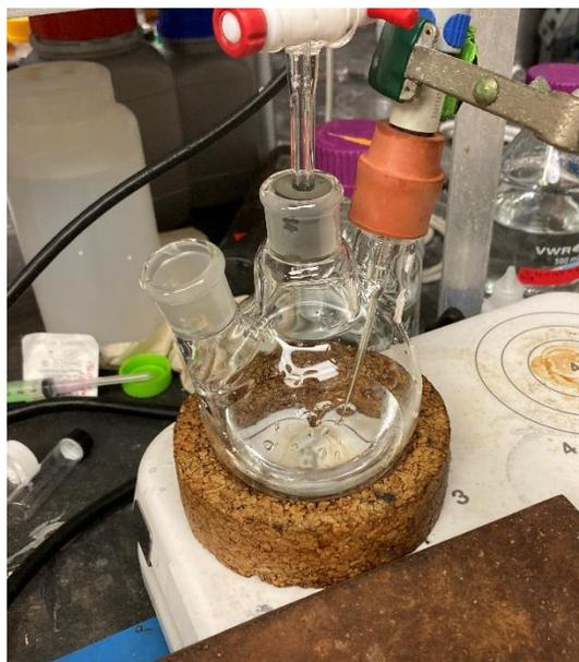
**Fig. B.12.** Three-neck flask used for silane titration. The center neck connects to a burette administering dilute 80 mM HCl; the rightmost neck connects to the pH meter. The leftmost neck, unused in the image, was connected to a condenser for measurements at 80°C.
