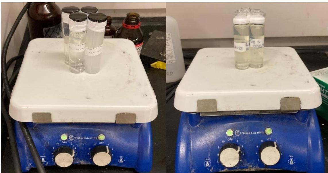
**Fig. A.4.** Left: nanoparticle condensation reaction of GPTMS and NexSil 6. While the temperature is not precisely controlled, we get excellent repeatability with this method. Right: evaporation of methanol after silanol condensation (also GPTMS and NexSil 6, but from a different batch).
