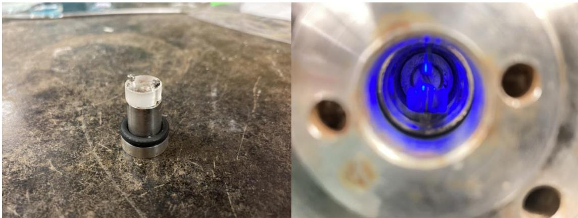
**Fig. B.10.** Left: specially-cut glass piece screwed in place on a mount. The mount plugged into the bottom of the high-pressure vessel, sealed with an o-ring. Right: view of glass piece in the direction perpendicular to the camera. The inlet line can be seen hovering closely above the glass surface.
